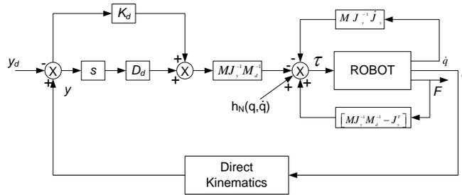
**Figure 6 . Impedance Control Block Diagram**
