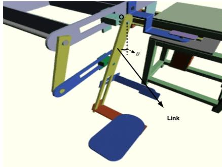
**Figure 7 . Knee link of robot manipulator**
