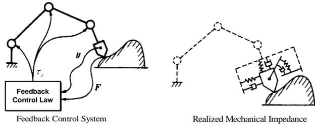
**Figure 5 . Active Impedance Method**
